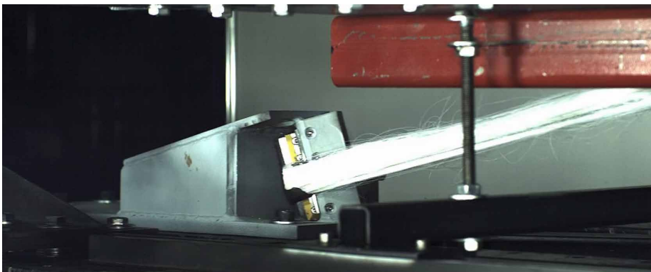
Development test 90° arrangement with redirection at a sharp edge
