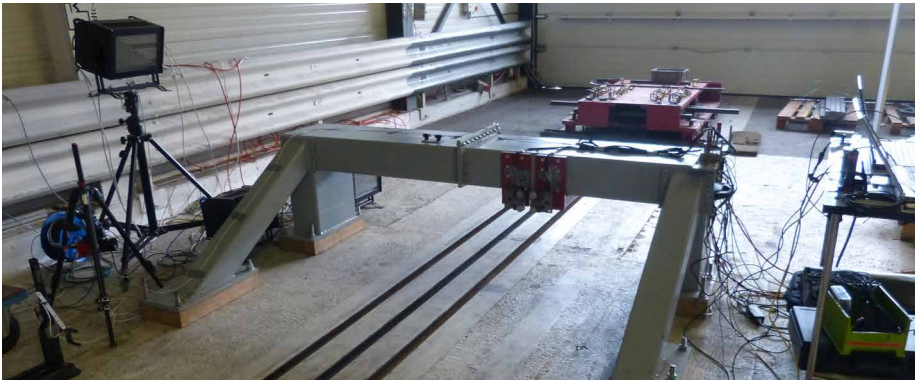
Raised test rig for angle adjustment and high-speed video setup
