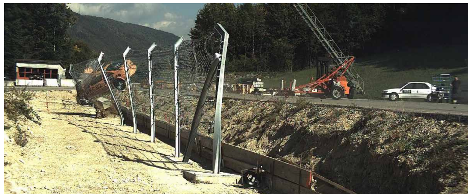
Rear view of a vehicle test on a stationary spectator protection fence
