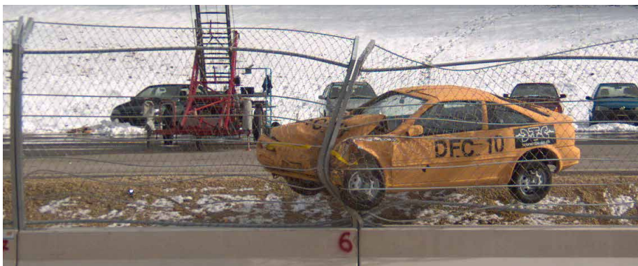
Vehicle impacts spectator protection fence at 122 km/h
