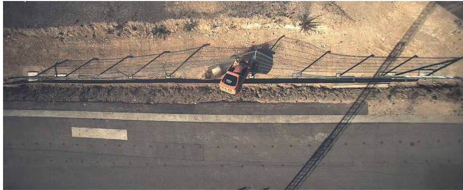
Top view of a vehicle test on a stationary spectator protection fence
