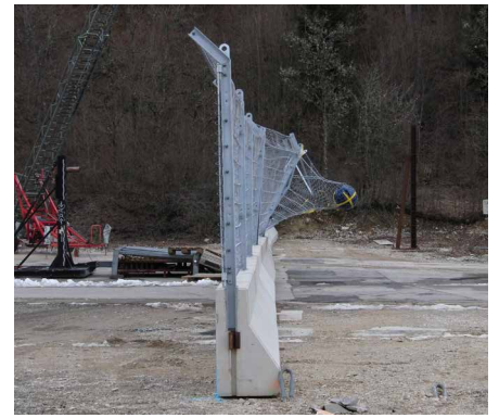
Side view of a sphere throwing test on a mobile spectator protection fence
