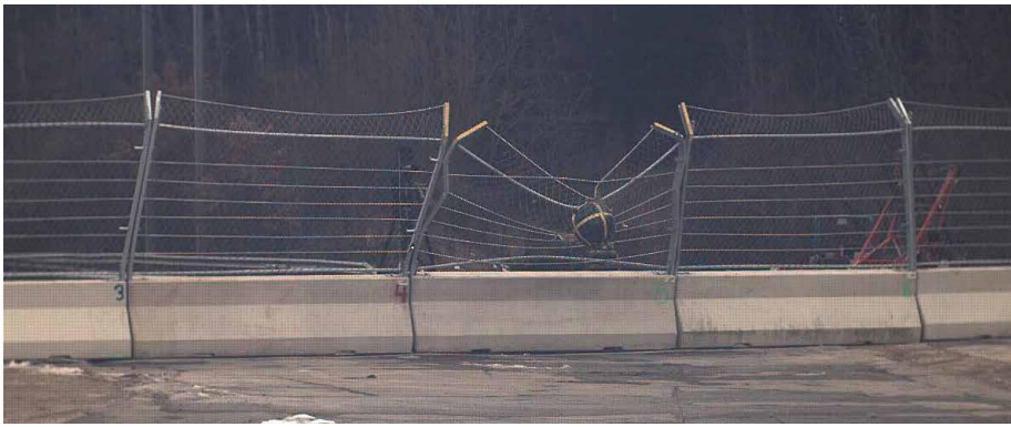
Rear view of a sphere throwing test on a mobile spectator protection fence
