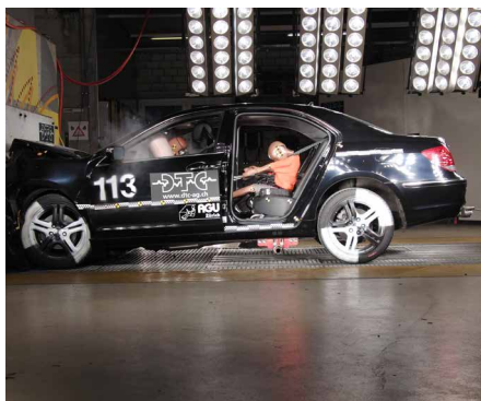
Frontal collision against a rigid barrier
