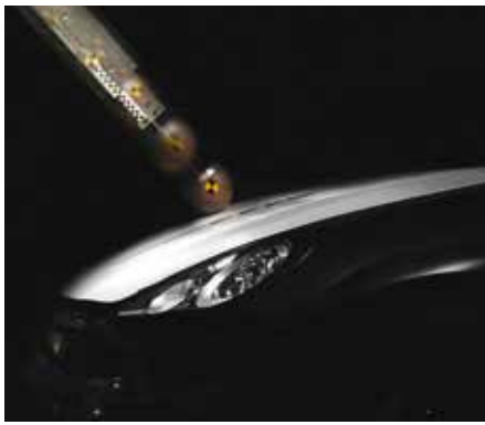
Head impactor shortly before impact
