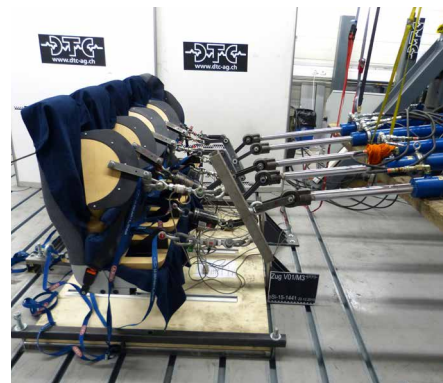
Quasi-static set belt anchor test
