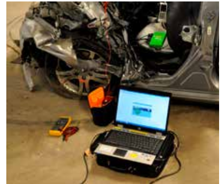
Read-out of event data in the control device (Bosch CDR)
