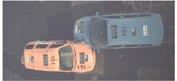
Fig. 15 The two longitudinal bars do not participate in the collision
