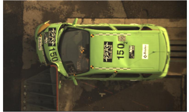
Fig. 11 The left longitudinal bar doesn't hit the barrier
