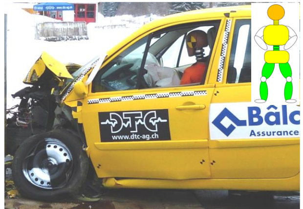
Fig. 33 Passenger compartment after IIHS small overlap Crash with reduced velocity DTC 149
