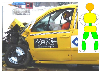
Fig. 35 Driver compartment after IIHS small overlap crash with reduced velocity DTC 149
