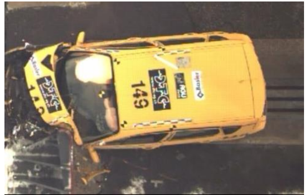
Fig. 20 Blocking of the compartment with the barrier
