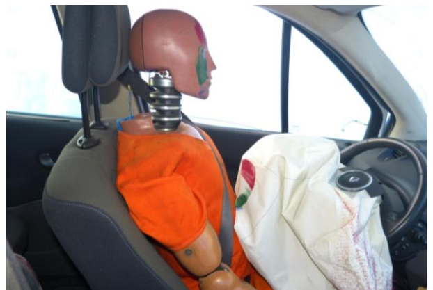
Fig. 18 Dummy head tracks on the airbag
