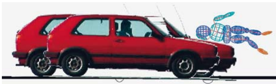
Simulation of a pedestrian accident by means of the multibody system (MBDEF)
